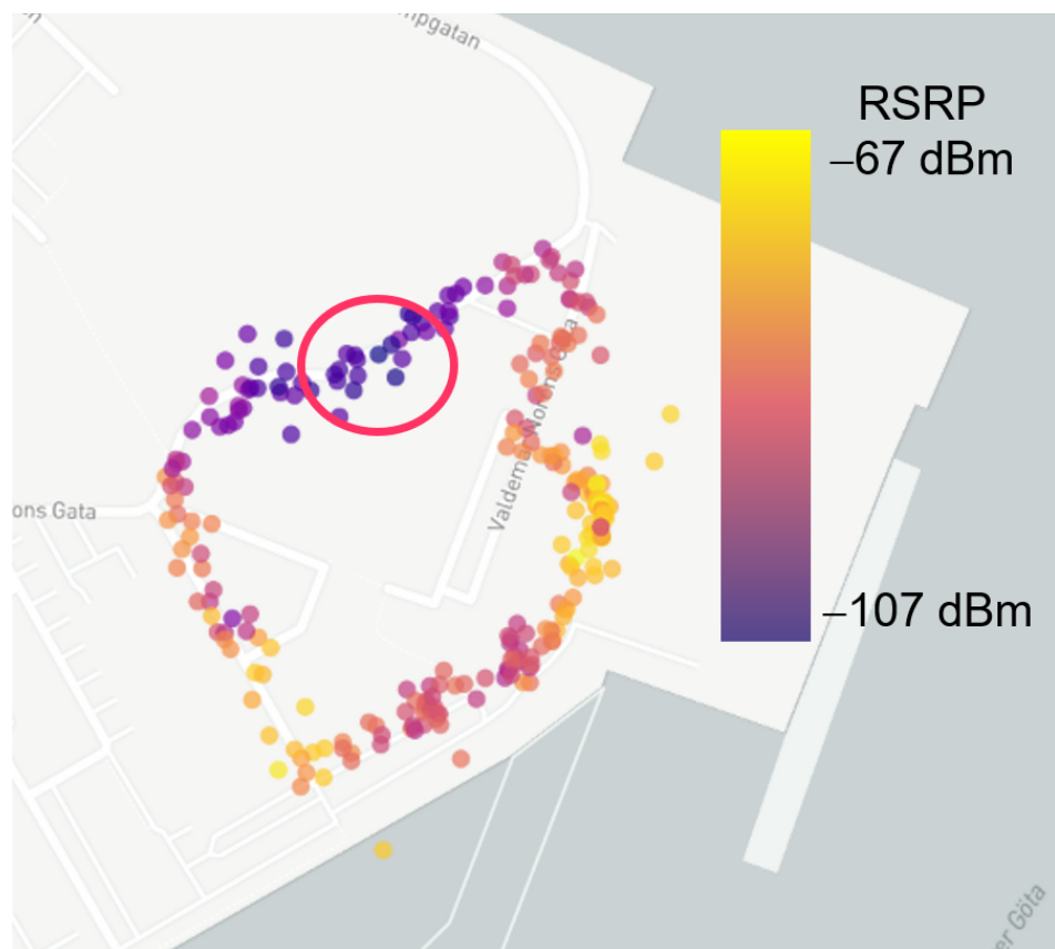
Figure 8. Reference Signal Received Power (RSRP) primary cells. Points of interest are circled in red.
